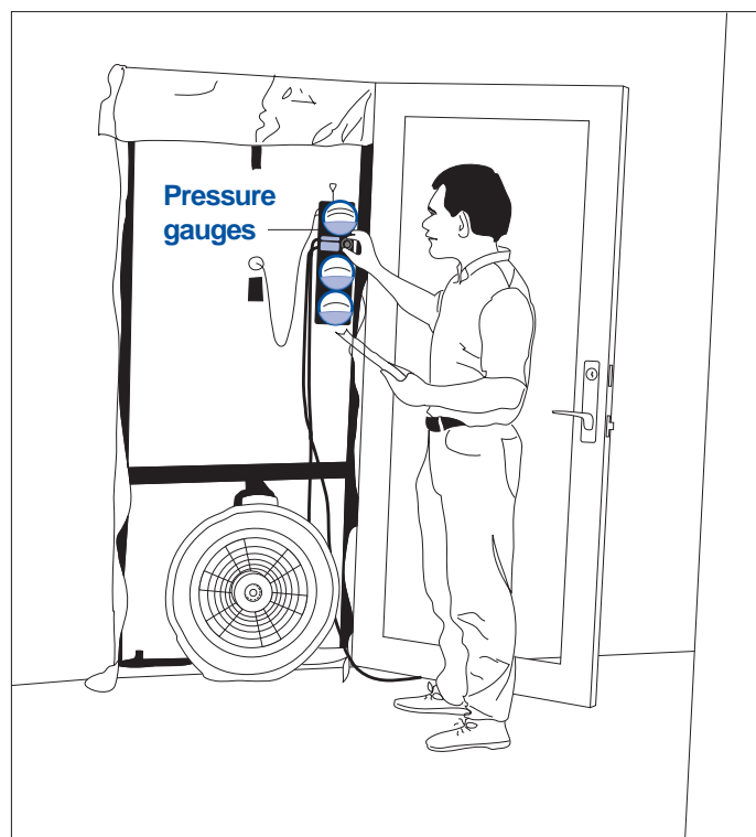
Figure 1-14 - Blower door for testing air leakage.
